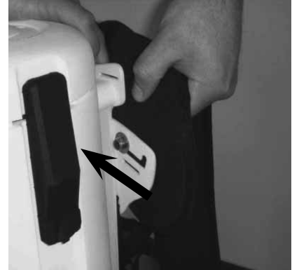
Adjustment of strap position on support plate
